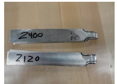
Figure3: Reduced Section specimens after tension
