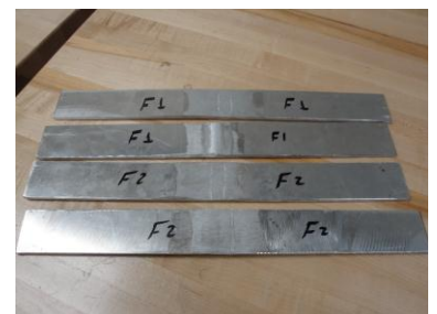
Figure4: Bending test specimens before bending
