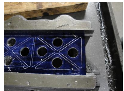
Drilling holes in the Vertical support
