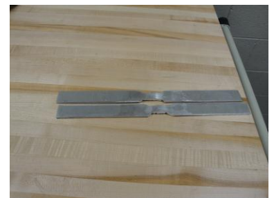
Figure2: Reduced Section specimens before tension
