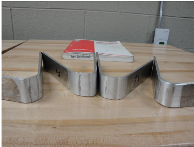
Figure5: Bending test specimens after bending
