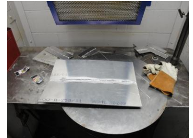
Figure1: Groove weld testing plate
